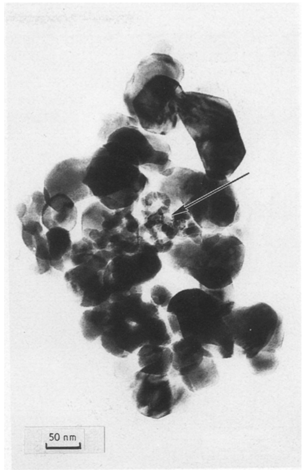
Figure 13 Small 10–30 nm amorphous particles (arrowed) between large 100 nm crystalline particles calcined at 600 °C for 2 h.
